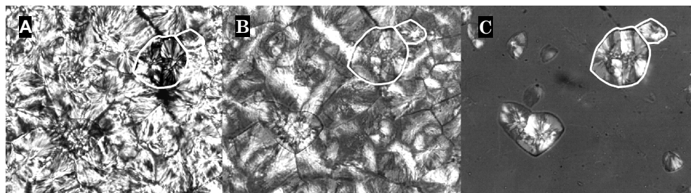
Figure 4.2. A polypropylene sample (ZN) nucleated with 0.01 wt.% CaSub, crystallized at 133°C, cooled to 110°C, and subsequently heated to 169°C at 10 °C/min. A, B, and C at 110, 158, and 169°C, respectively.
